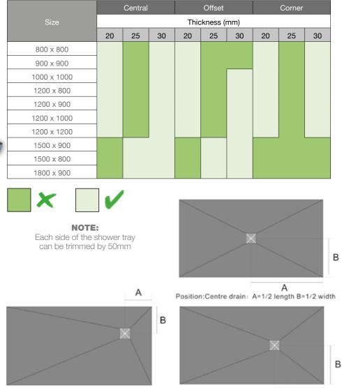
Normal Position:Corner drain: A=B=260mm
